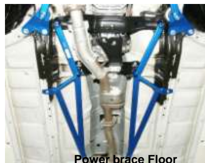
Power brace Floor
