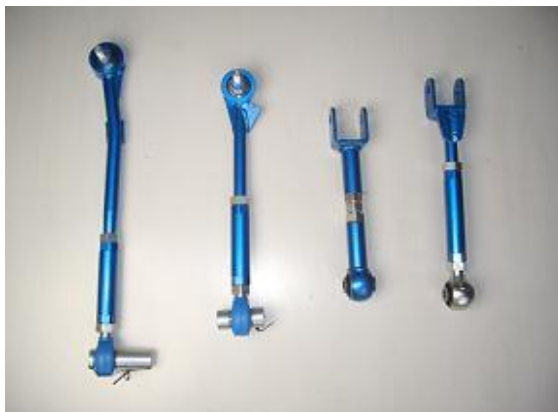
from Left Pillow tension rod, Front Pillow lower arm, Rear Upper arm, Rear Toe control rod
